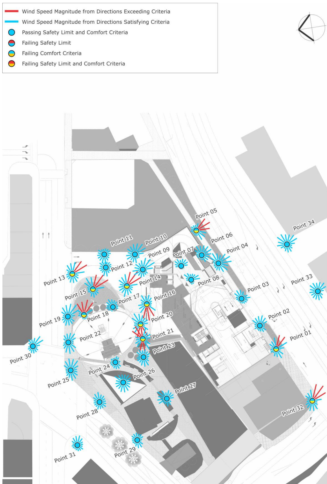
Figure 10a: Wind Tunnel Results – Ground Level Plans (Proposed Surrounds Case) (results shown without treatments applied)
