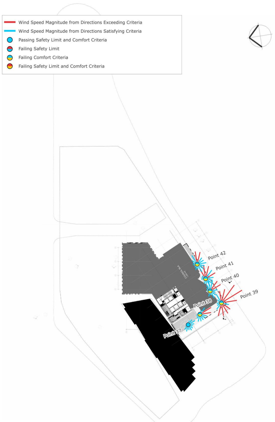
Figure 11c: Wind Tunnel Results – Level 04 Plan (Future Surrounds Case) (results shown without treatments applied)
