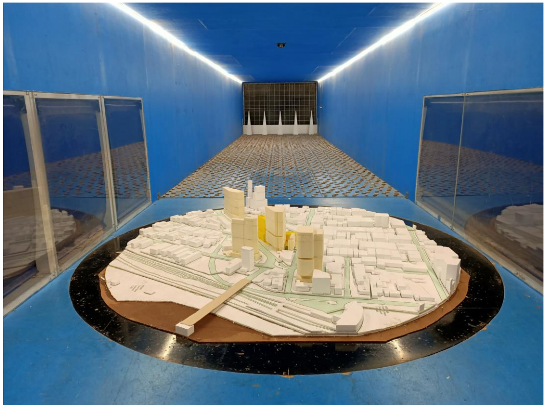
Figure 5b: Photograph of the Wind Tunnel Model – Future Case (view from the east)
