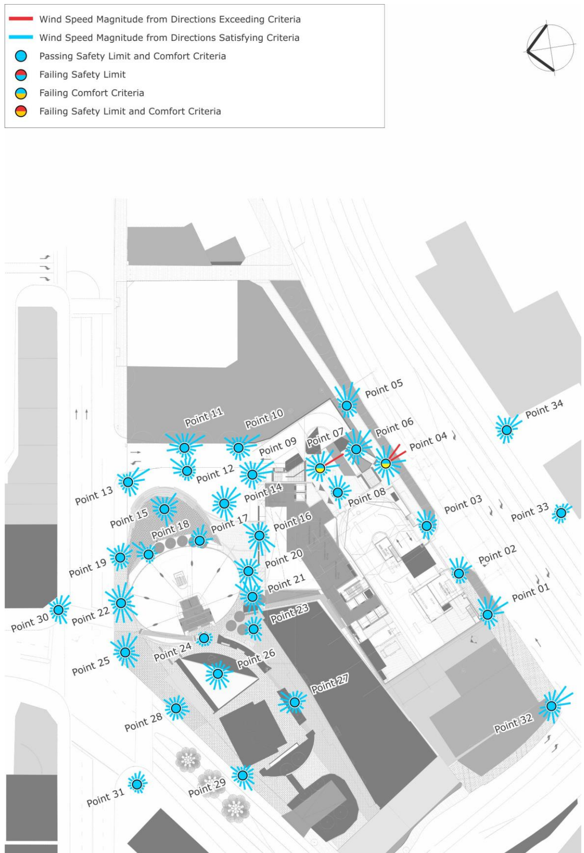
Figure 11a: Wind Tunnel Results – Ground Level Plans (Future Surrounds Case) (results shown without treatments applied)
