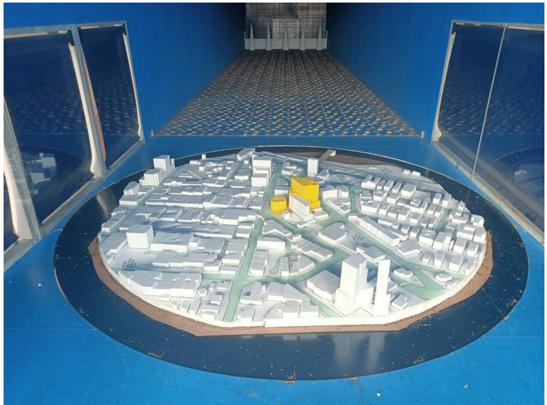
Figure 4d: Photograph of the Wind Tunnel Model – Proposed Case (view from the west)
