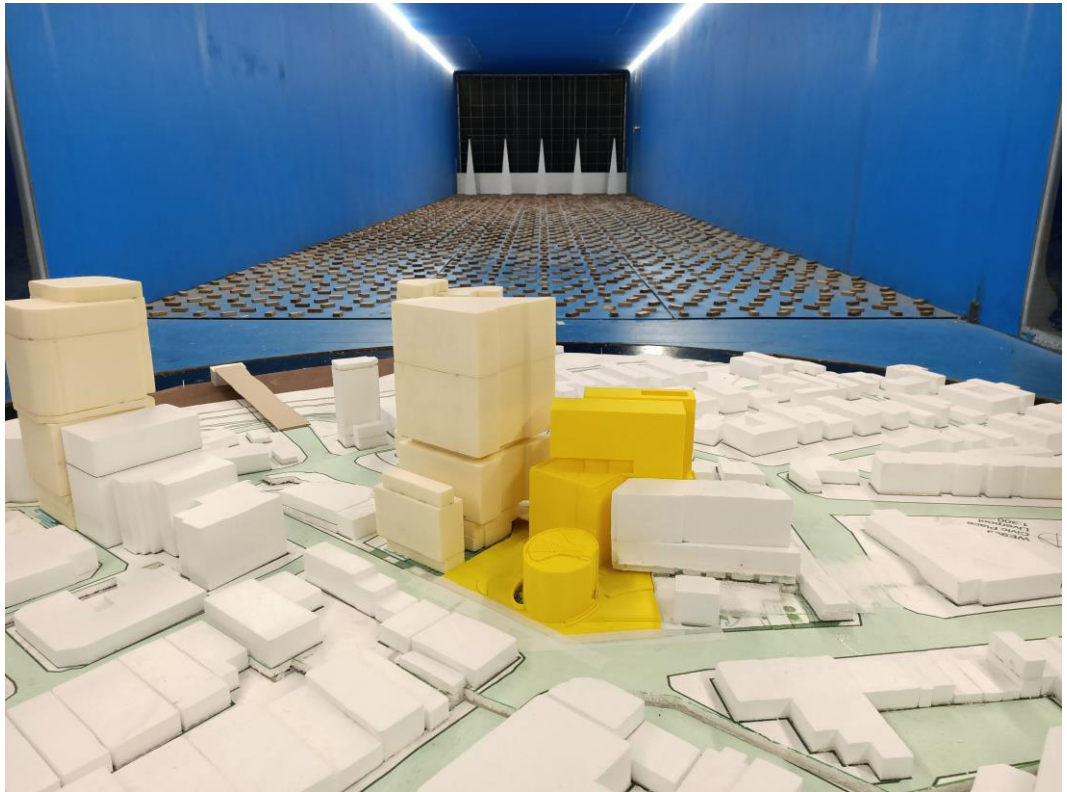
Figure 5e: Photograph of the Wind Tunnel Model – Future Case (view from the north-west)
