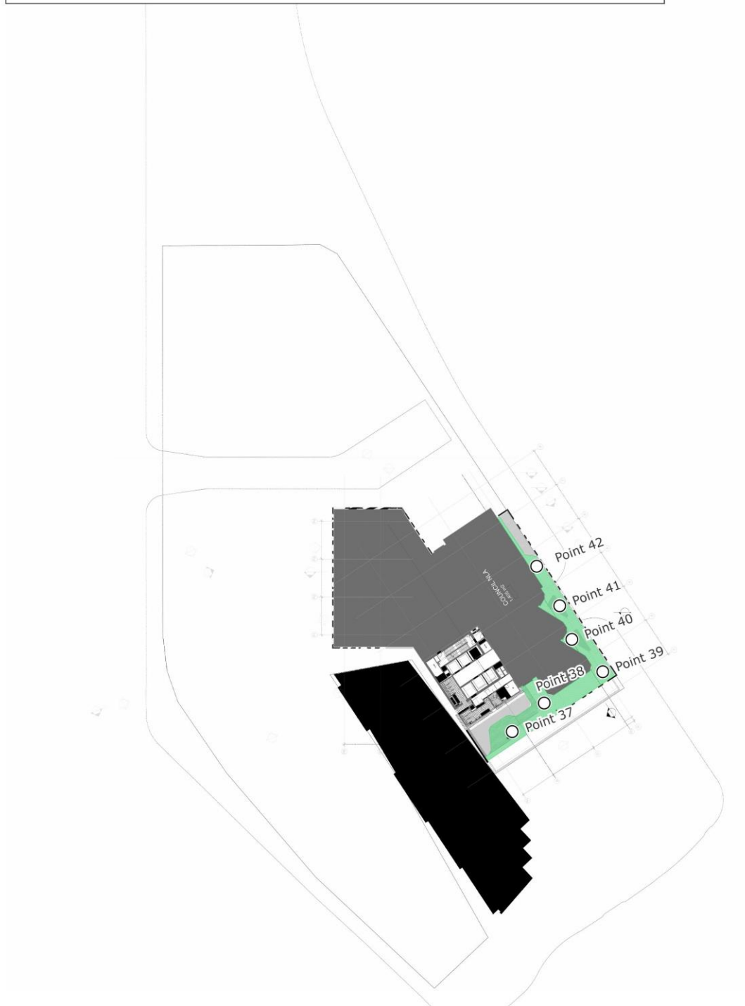
Figure 9c: Study Point Locations and Target Wind Speed Criteria Level 04 Plan
