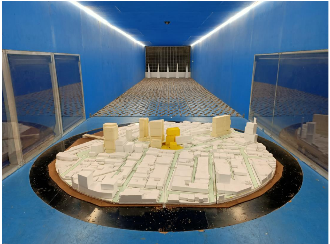
Figure 5a: Photograph of the Wind Tunnel Model – Future Case (view from the north)
