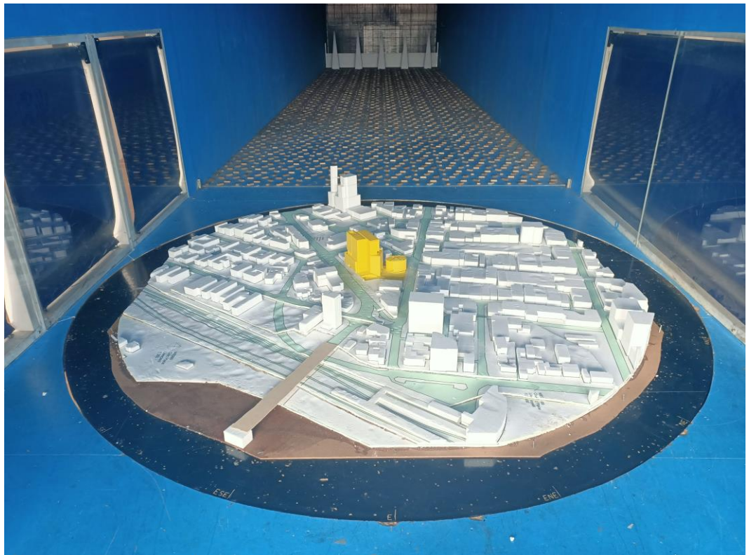
Figure 4b: Photograph of the Wind Tunnel Model – Proposed Case (view from the east)
