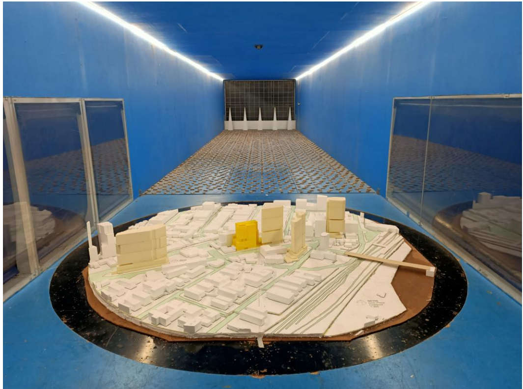
Figure 5c: Photograph of the Wind Tunnel Model – Future Case (view from the south)
