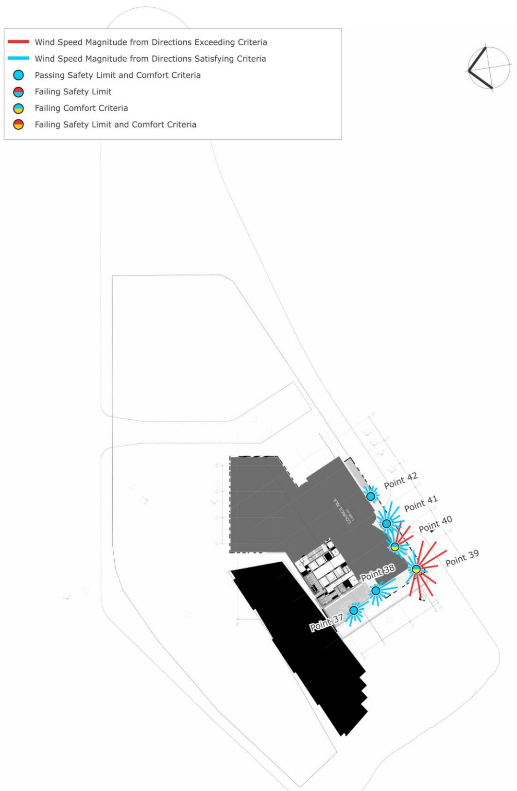
Figure 10c: Wind Tunnel Results – Level 04 Plan (Proposed Surrounds Case) (results shown without treatments applied)
