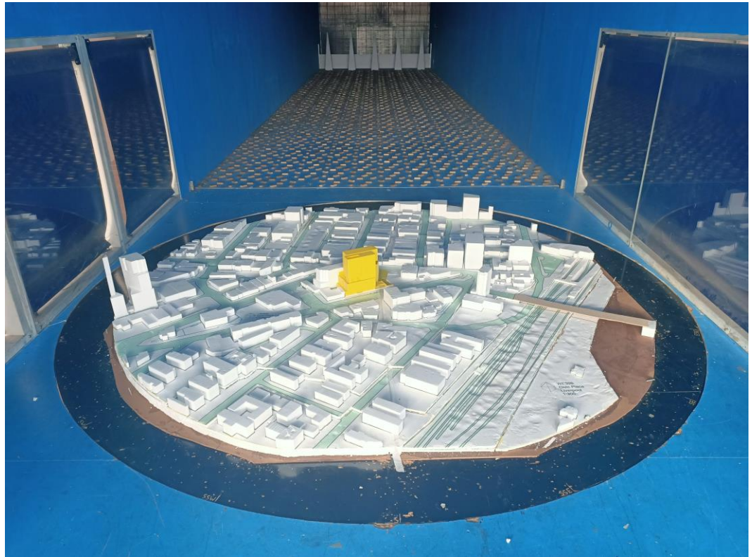
Figure 4c: Photograph of the Wind Tunnel Model – Proposed Case (view from the south)
